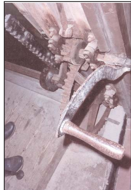
Winding mechanism for sluice
