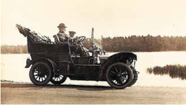
A 1908 Victoria tourer with a 10/12hp Fafnir engine manufactured by Victoria Motor Works (Godalming) Ltd
